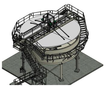
The sludge rake operates by pushing lime solids along the bottom of the tank using 10 GR316 SS blades with neoprene squeegees. The blades are angled so that sludge is pushed to the centre of the tank, where it can be recirculated or wasted.
