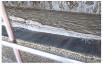
Fats and grease removed from the DAF surface
