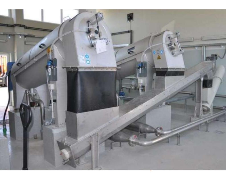
■ The HUBER ISP is ideal for dewatering primary sludge from DAF systems and clarifiers or biological sludge generated by industrial wastewater treatment plants.
