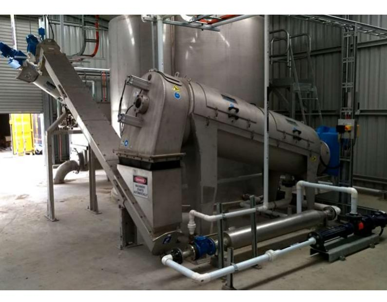
The Screw Press system is the hardware of the dewatering system but it is surrounded by expertly designed ancillary components that ensure the overall treatment system is simple to operate and maintain with optimum performance
