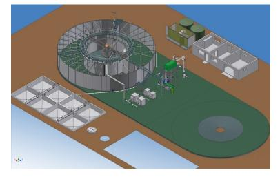
To facilitate site installation the entire structure of the activated sludge process was fabricated using the Roadtrain® bolted design.
