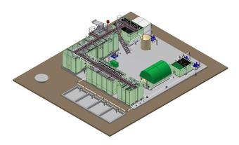
Effluent from the RBC unit flows to the deoxygenation tank, which allows the residual oxygen from the RBC reactors to be dissipated. This deoxygenated sewage is then recycled to the anoxic tank, where the nitrates generated in the RBC reactors is reduced to nitrogen gas.
